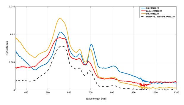
**Figure 2.** Examples of oil spectra compared with water spectra. Note the characteristic peak of reflectance at 0.705 micron, due to *Lemna obscura*, a floating vegetation typical of Lake Maracaibo.
