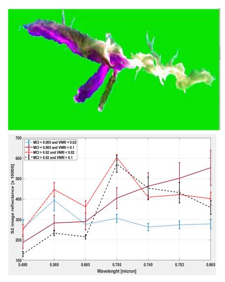
**Figure 7.** (**Upper**): RGB image of the 27 February 2017 obtained by combining MCI map (R), VNRI (G), and S2 band 4 (B). (**Lower**): Spectral profiles corresponding to different conditions of the water in the lake.
