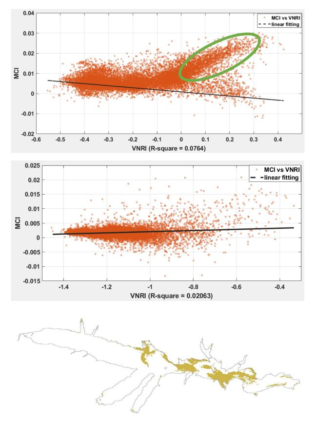
**Figure 5.** Comparison between VNRI and MCI values to check the correlation between indices. Plots are based on the analysis of the S2 images of 27 February 2017 (**top**) and 01 July 2021 (**middle**). (**Bottom**) image shows the area of the lake corresponding to the pixel values of the ascending branch (pixel values enclosed in the green ellipse) of the top plot.
